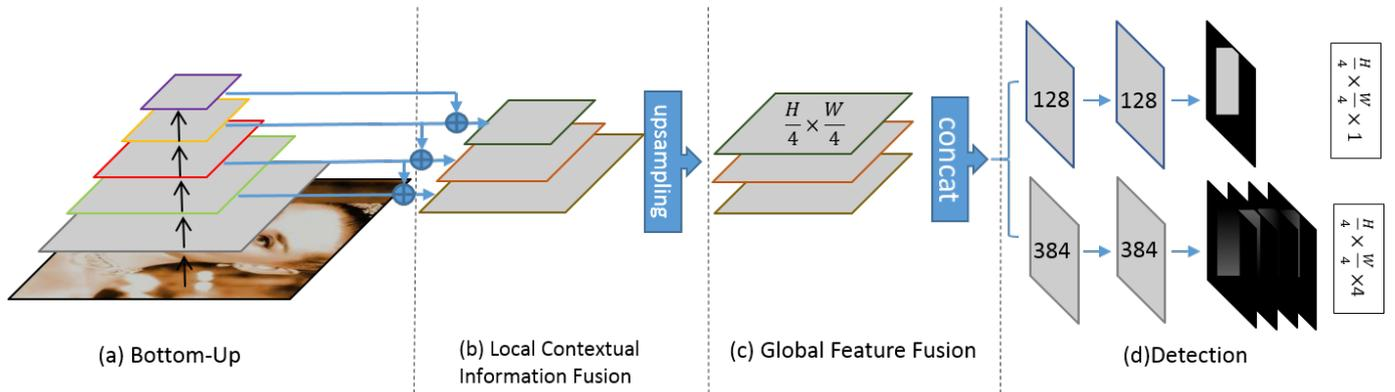
Fig. 2. The proposed detection system backbone on top of a feed-forward VGG architecture, combined with four major part: (a) Bottom-Up Pathway. (b) Local Contextual Information Fusion, merged local contextual information by addition. (c) Global Feature Fusion, adjust all features to the same resolution and merged in series. (d) Detection, based on fused feature we use two independent task related network to predict pixel level classification and bounding box regression.
