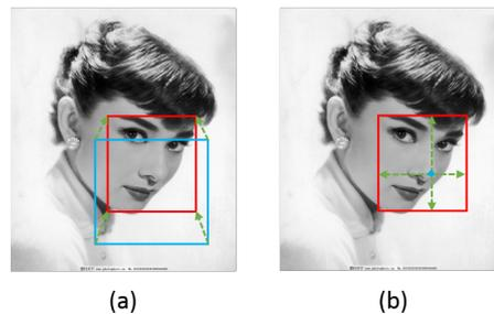
Fig. 1. A visual explanation shows the difference of anchor-based and anchor-free methods. The red bounding box is the ground truth, the blue bounding box is a predefined anchor, and the green lines are the offsets. (a) The anchor based methods predict the offsets based on predefined anchor. (b) The anchor-free methods directly estimate the offsets of a point to its outside boundaries.
