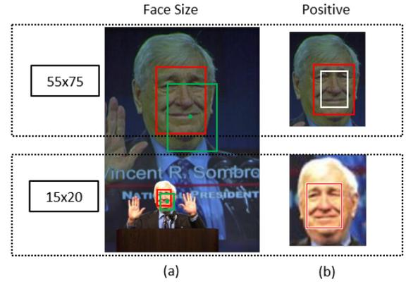
Fig. 4. An illustration of scale aware balance sampling, two faces are annotated with red box in the same image. Green boxes are templates in green point position. Pixels within white boxes are positive examples. The sizes are controlled by  $\delta_{pos}$ .
